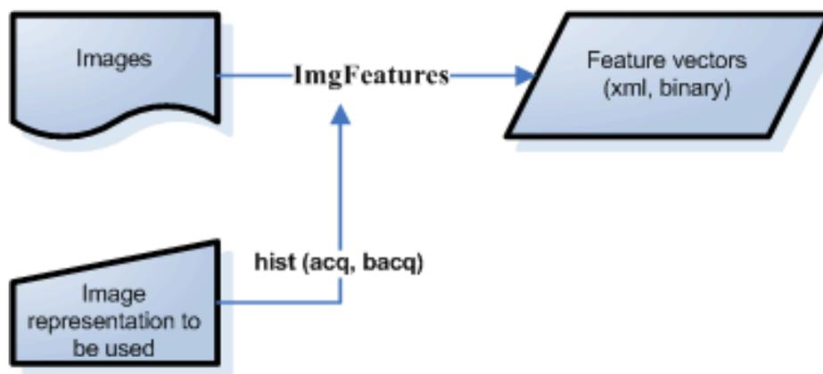
**Figure 2.** Architecture of the system for representing images as feature vectors based on a quantized color space using histograms (hist), autocorrelograms (acq), or banded autocorrelograms (bacq).
