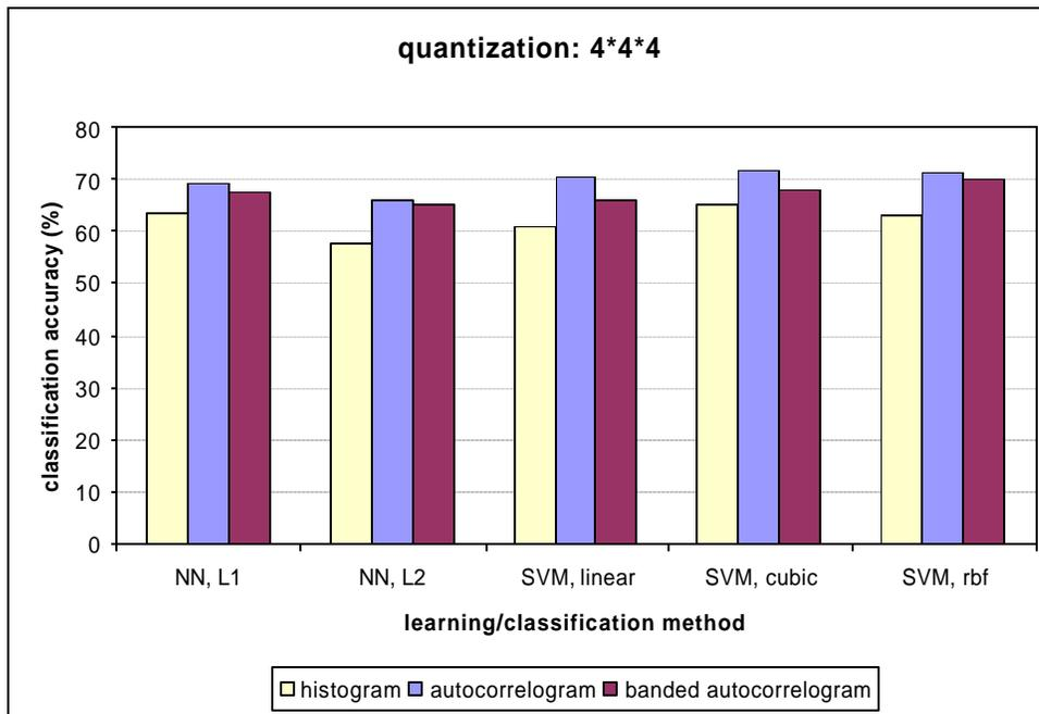
**Figure 3.** Results of the experiments comparing different combinations of image representation, and classification method using colorspace quantization: 4x4x4.
